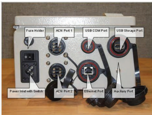
Figure 4. Photos of the prototype PIT tag system with one MC and two updated ACNs. We drew lines to represent the antenna cables and communication lines that connect the two parts. Each ACN would also need power to energize its antenna.
